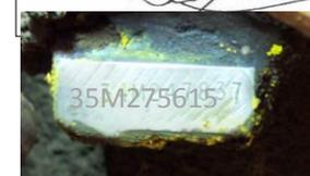
The stamping is on the small smooth pad on the block and is seen from the driver's side. It is below the cylinder head, behind the power steering pump and difficult to see.
