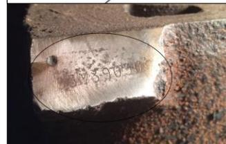
The stamping is on the small smooth pad on the block and is seen from the driver's side. It is below the cylinder head, behind the power steering pump and difficult to see.
