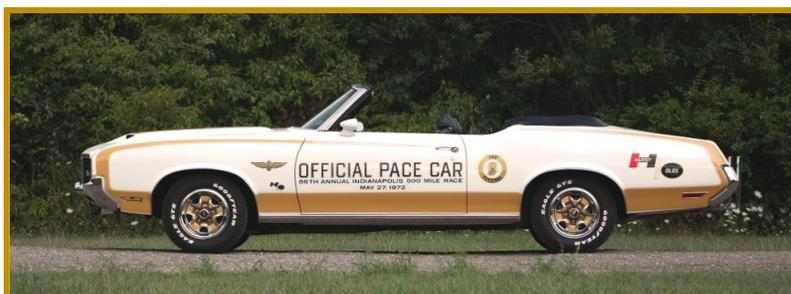
Hurst Performance did their portion of the 1972 conversion at the Demmer facility in Lansing, MI. It consisted of applying the unique gold stripes on the hood, sides and trunk lid, apply three exterior Hurst/Olds emblems and Indy decals if ordered; install a Dual-Gate shifter in the original Oldsmobile console; and apply the special Indy 500 decal and emblem to the glove box door.
