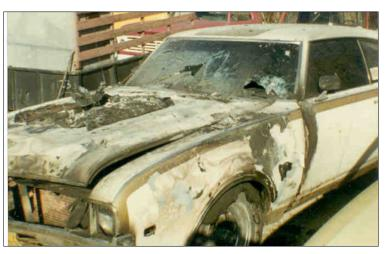
The vast majority of vehicle fires start in the engine compartment usually due to a fuel leak caused by a stuck carburetor float, cracked fuel line, or a loose connection etc. It is rather common for the fuel filter fitting to be stripped or left loose on the Oldsmobile Quadrajet. An electrical short is probably the next most common cause.
